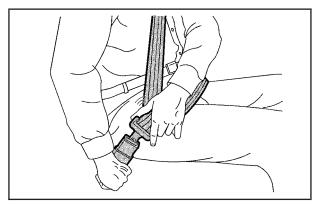
Pick up the latch plate and pull the belt across you. Do not let it get twisted. 4. Push the latch plate into the buckle until it clicks.
